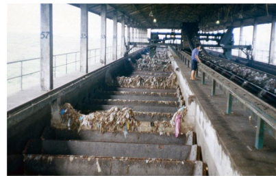
John Thompson composting plant built on the dumpsite around 1960, sold on strength of one operating plant in Jersey (UK) (Breidenbach, 1971). Incoming mixed waste pulverized in a hammermill, then conveyed to top of six-floor building; waste remained on each floor for one day, then released mechanically to next floor down (the aeration process). 'Composted' waste matured for some months before being sieved in a compost finishing plant. Unclear how far the plant had ever been successful; by 1983, still in use but compost no longer sold.
