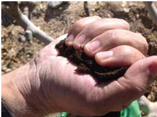
Figure 4.7. Field Test Demonstrating the Presence of Adequate Moisture in the Compost.
