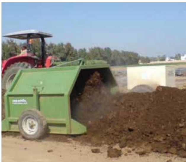
Figure 4.4. Windrow Turner Machine.
