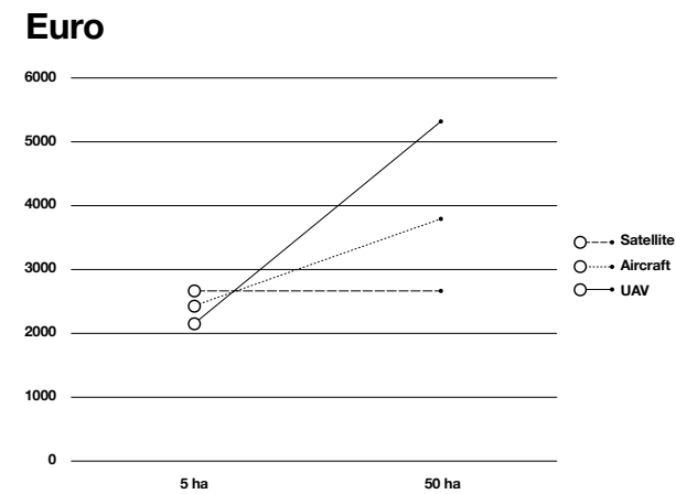
FIGURE 22: PLOT OF CATEGORY COSTS (EURO) FOR SATELLITE, AIRCRAFT AND UAV PLATFORM, CONSIDERING A 5-50 HA MAPPING AREA 95
